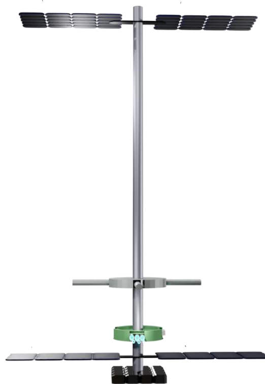
Step 2 – Spokes and MPA will be assembled from the construction shack.
